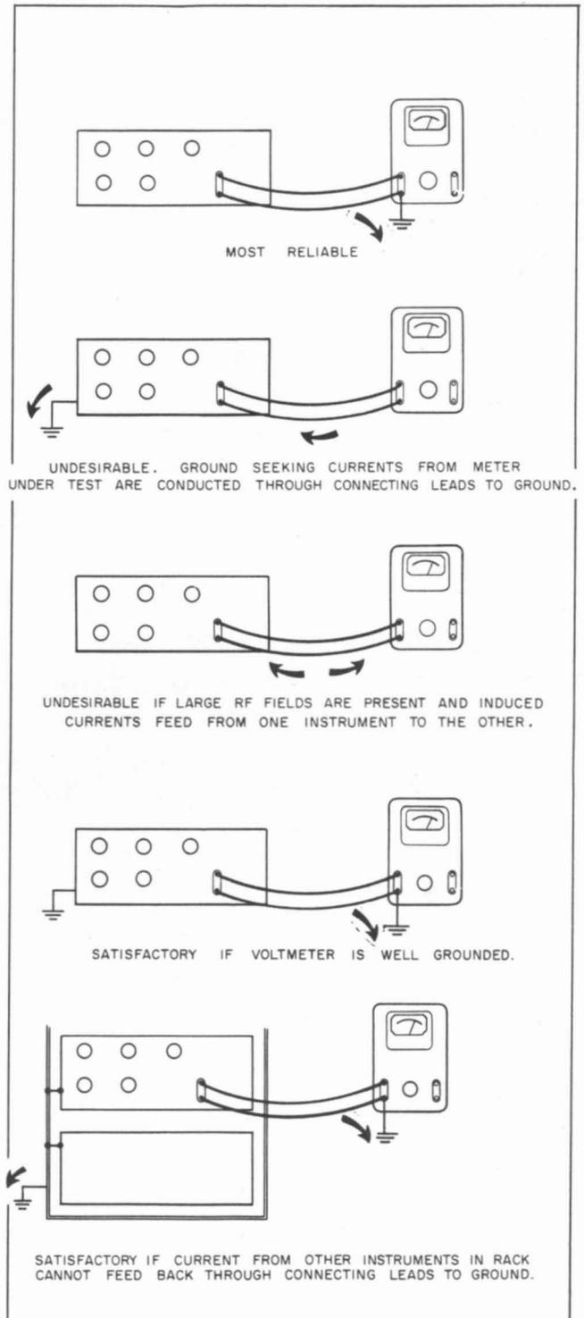
Figure 2-2. Desirable and undesirable arrangements for grounding instrument chassis when using the Voltmeter Calibration Generator
