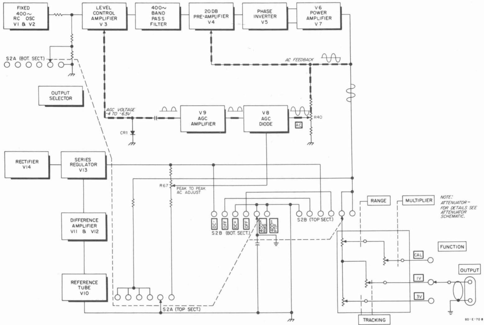
Figure 3-1. Block Diagram Model 738A
